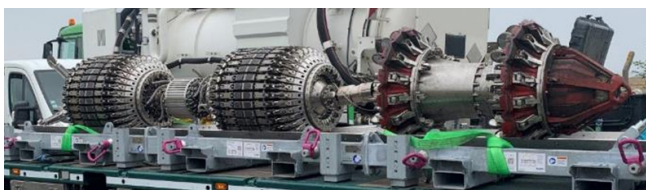
Figure 3. Picture of an EMAT-C Ultra tool at job site before launching.
