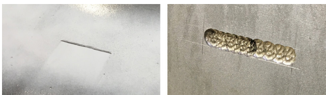
Figure 11. Example of a synthetic crack (made visible by MPI) and a synthetic sharp-edged corrosion.
