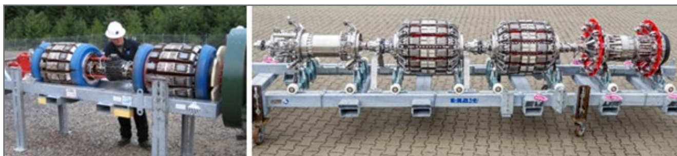
Figure 2: Comparison between EMAT-C tools from around 2006 (left) and 2023 (right)
