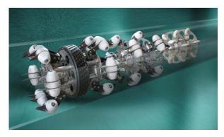
The bi-directional capability is achieved through adapting the sensor-carrier, electronics and data-storage modules into lightweight low-friction modules and combining them with a powerful wheel-driven crawler. The tether supplies electrical power to the tool, bringing the collected data to the control unit at the launching site. This allows for remote steering of the crawler and acts as a means of recovery in emergencies.
