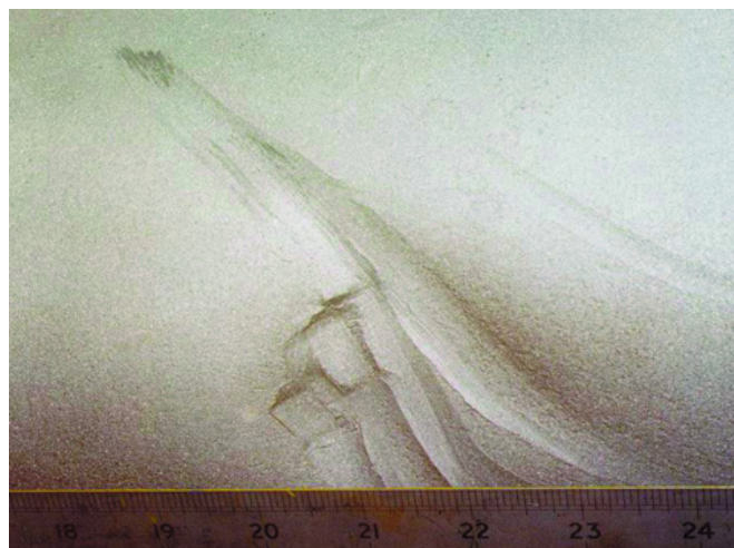
Figure 2. A typical dent-gouge combination.
