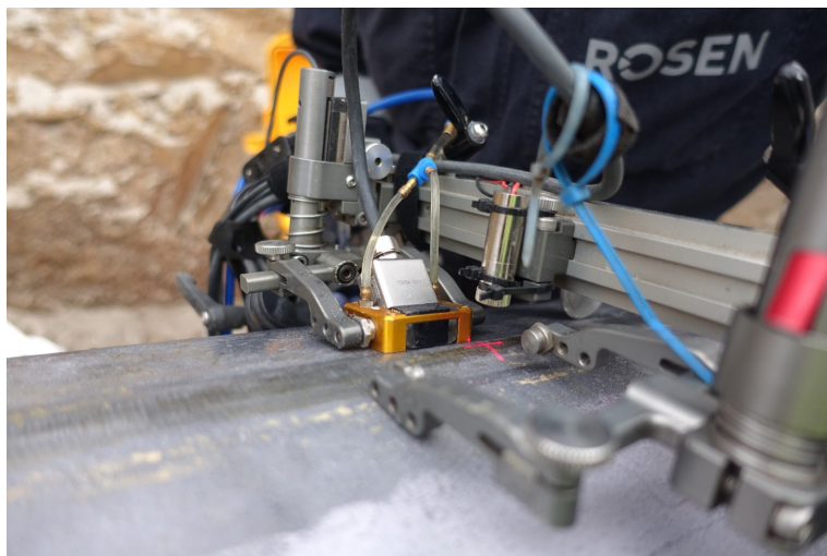
Figure 3. PAUT inspection of a long seam.
