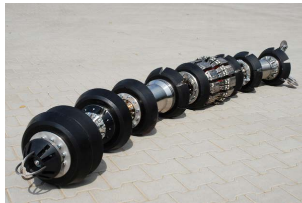
ATEX-compliant 12" Magnetic Flux Leakage Metal Loss ILI tool
