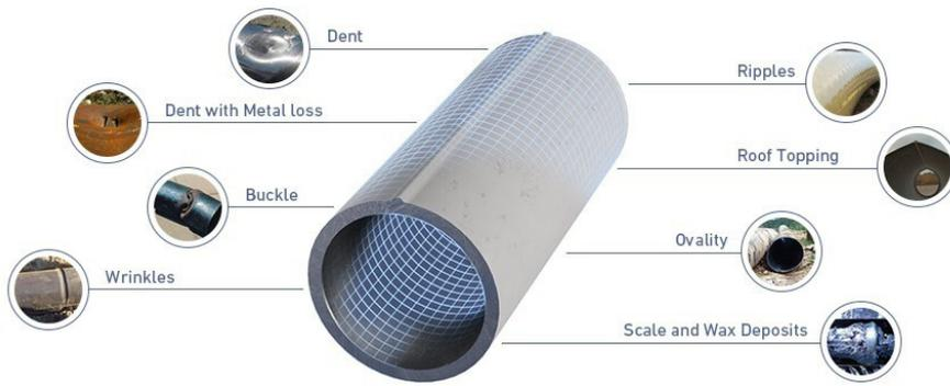
Figure 2. Geohazards can change the shape of a pipeline and may create local features, such as dents, buckles, ovalities and bending, all with potentially detrimental effects on the pipeline's integrity.
