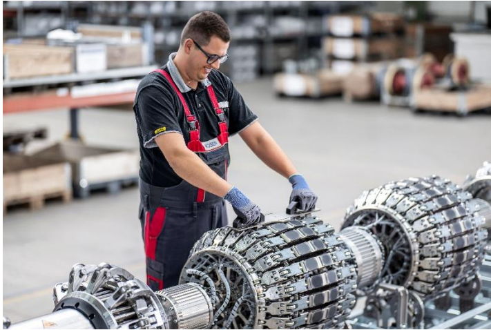
Caption: Technician working on RoCD EMAT-C Ultra tool.
