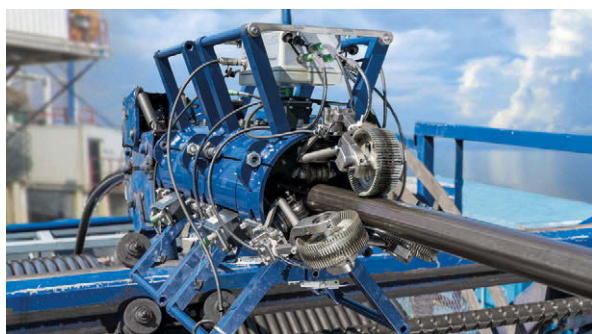
ACIM inspection head clamped on coiled tubing during offshore operations
