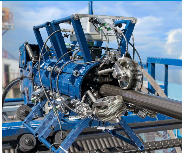
ACIM inspection head clamped on coiled tubing
