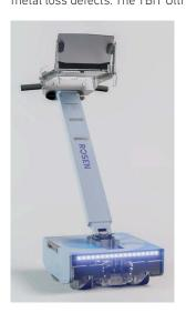
maximum coverage of the tank floor by using a remote-control tank floor scanner for difficult-toaccess areas (e.g. under piping or heating coils). In addition, a dedicated Blind Zone Scanner for areas that otherwise remain uninspected due to the physical limitations of the floor scanner significantly reduces the risk of missing relevant metal loss defects an areas normally not being covered by floor scanners.
