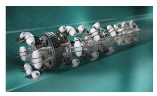
The bi-directional capability is achieved through adapting the sensor-carrier, electronics and data-storage modules into lightweight low-friction modules on wheels and combining them with a powerful wheel-driven crawler. The tether supplies electrical power to the tool, bringing the collected data to the control unit at the launching site. This allows for remote steering of the crawler and acts as a means of recovery in emergencies.
